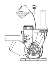
When used of the suction lift, filling the inlet pipe and pump with water to reduce lifting time. Please install a foot valve; and, please remove the check valve to filling up the water and assemble it back once it has do
