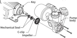
E.Press the stationary part of the shaft seal firmly into the pump head.
