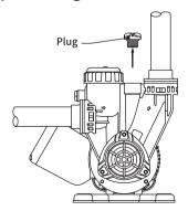
② When the water source's pressure is insufficient, please unscrew the priming plug and fill up the pump chamber with water, then, screw it on.
